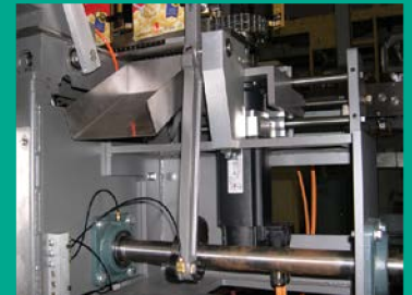
Servo control used for increased precision
